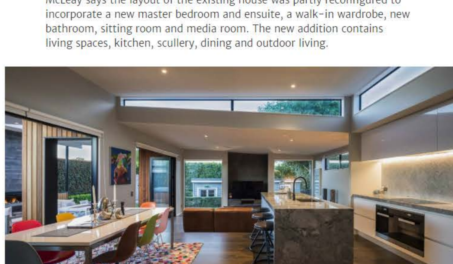
Cleerestory windows bring in extra light and allow glimpses of the tree canopy beyond.
